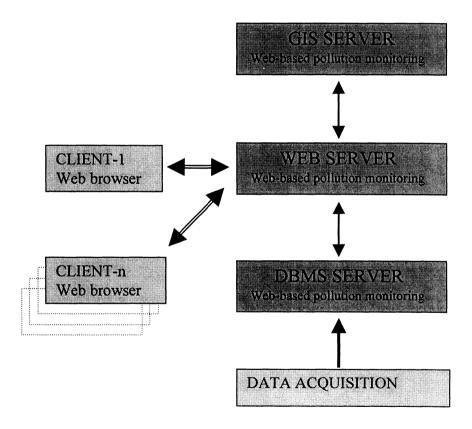
Fig.2 Pollution monitoring system architecture
