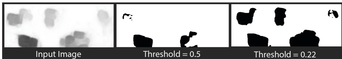
Fig. 2.4 Effects of probability threshold. A probability threshold of 0.50 means that the pixel is classified as class if the model is surer than 49.8 % that this pixel is a class pixel. A probability filter of 21.57 % means the model must be surer this value.
