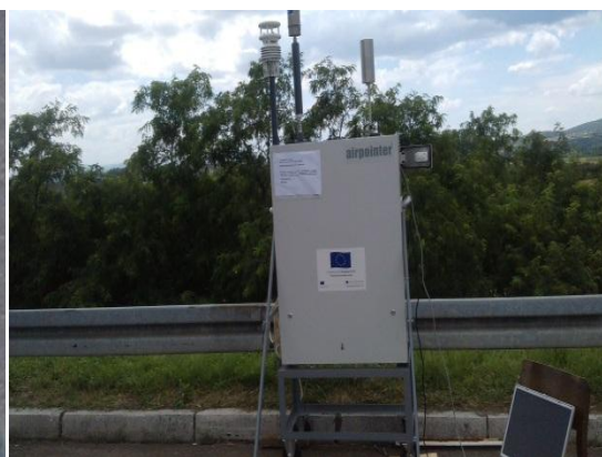
Figure 2. The measuring station "Airpointer®" at the measuring point – tollbooth Nais on highway E75
