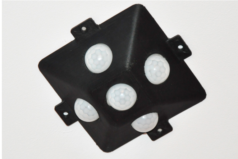
Fig. 1. Five PIR sensor IoT device.
