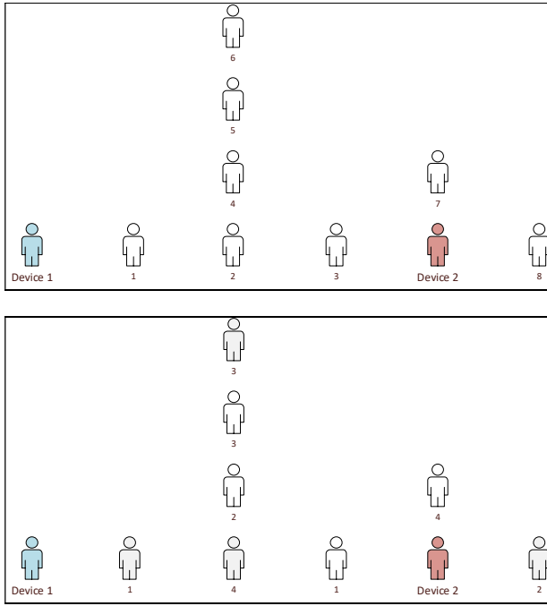
Fig. 4. The 8 configurations at the distance of 4m for scenario 2 (upper) and the 4 configurations at the distance of 4m for scenario 3 (lower)
