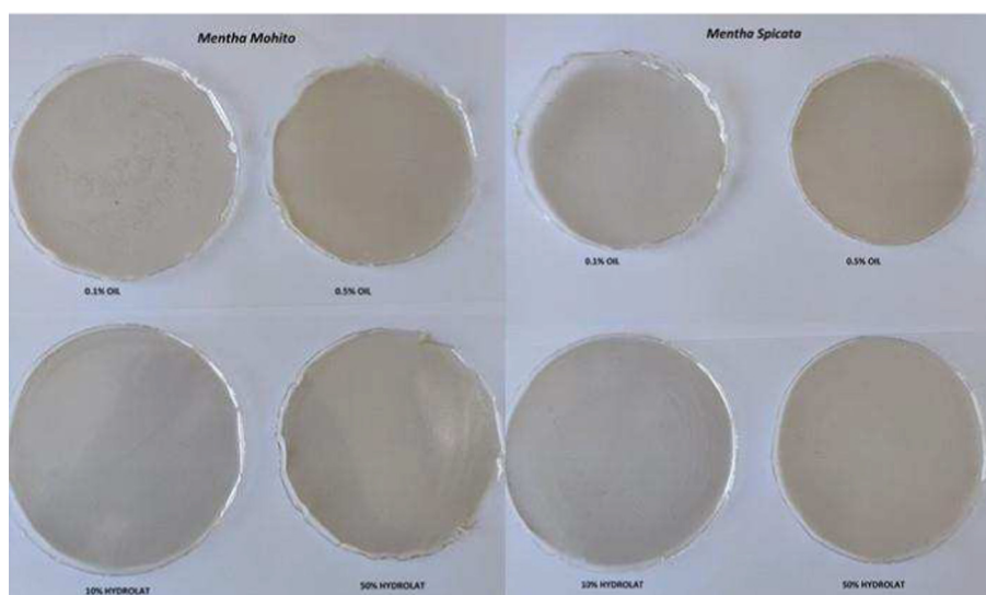
Fig. 1. Gelatine films with Mentha mohito and Mentha spicata oil (0.1%; 0.5%), in the first row, respectively; Gelatine films with Mentha mohito and Mentha spicata hydrolat (10%; 50%), in the second row, respectively
