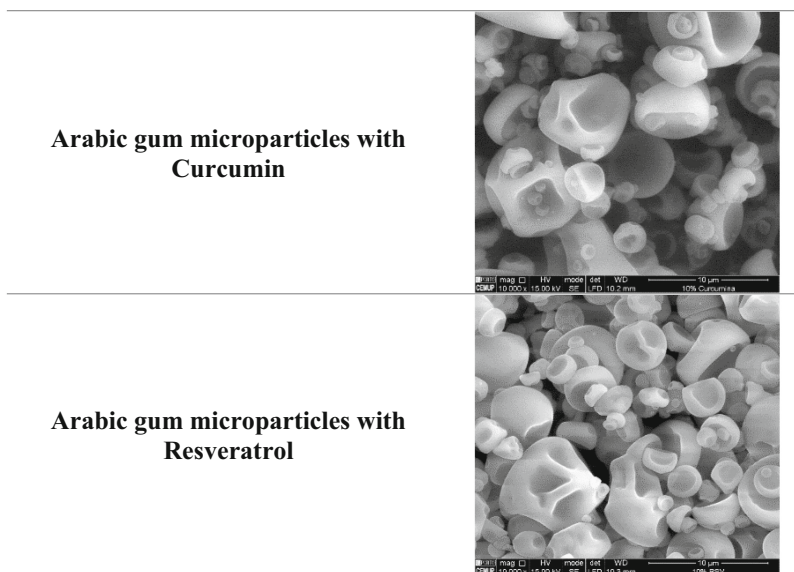
Fig. 5. SEM images of polyphenol (curcumin and resveratrol) microparticles prepared with arabic gum (10%) by emulsification+spray drying. SEM specifications: magnification of 10 000 ×, beam intensity (HV) of 15.00 kV, distance between the sample and the lens (WD) around 10 mm.
