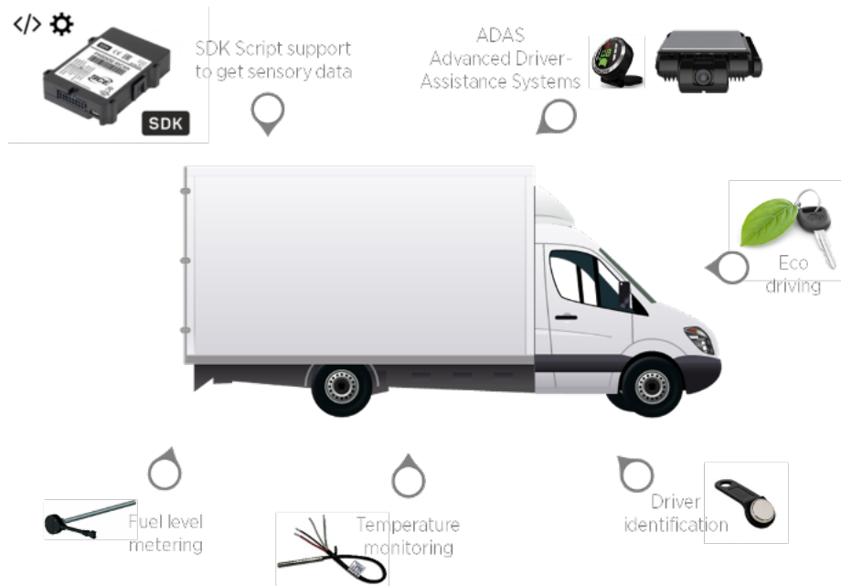
Fig. 1. Overview of devices and sensors used for research set-up
