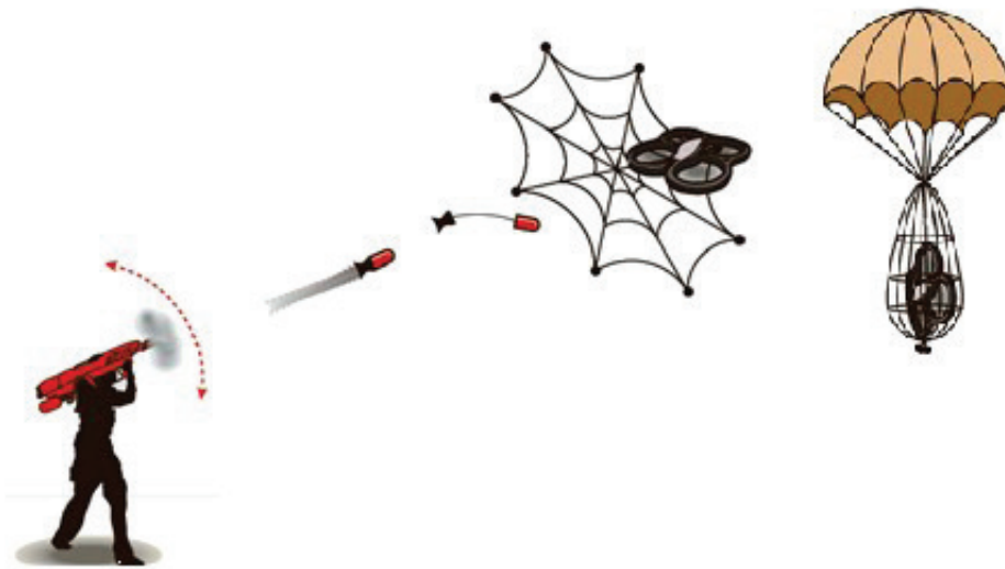
Figure 2: Principle sketch of SkyWall 100 ®
