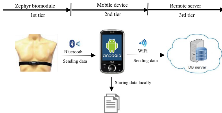
Fig. 1. Architecture of developed healthcare monitoring system
