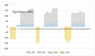
Figure 17. Generated and consumed power for 3 days operation
