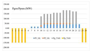
Figure 13. Generated and consumed power for the HPS on Fig.11
