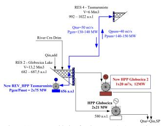
Figure 11. HPS considering for short term (ST) operation modes
