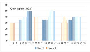
Figure 16. Turbine and pump flows for 3 days operation
