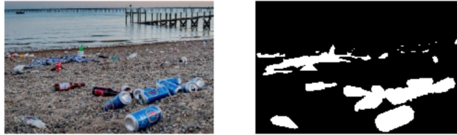
Fig. 3. An image from the dataset, next to its segmentation. The white segments represent garbage regions.
