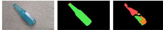
Fig. 6. Example of segmentation results for glass-based garbage class on the test set. Original image (left), Ground truth segmentation (Middle), Segmentation result (right)
