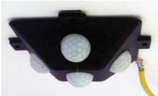
Fig. 2. Casing and sensor placement within the casing [6]
