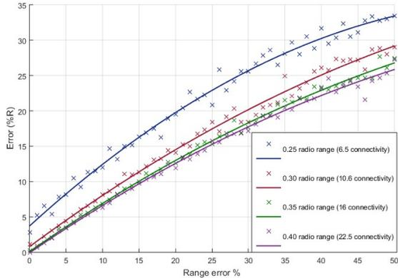
Fig. 5. Relationship between the radio range error and the average estimation error for different connectivity level
