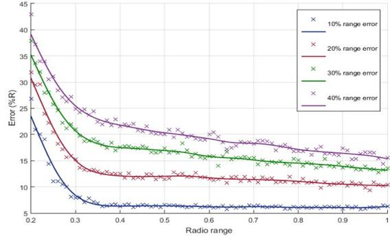
Fig. 6. Relationship between radio range and average estimation error for different radio range error
