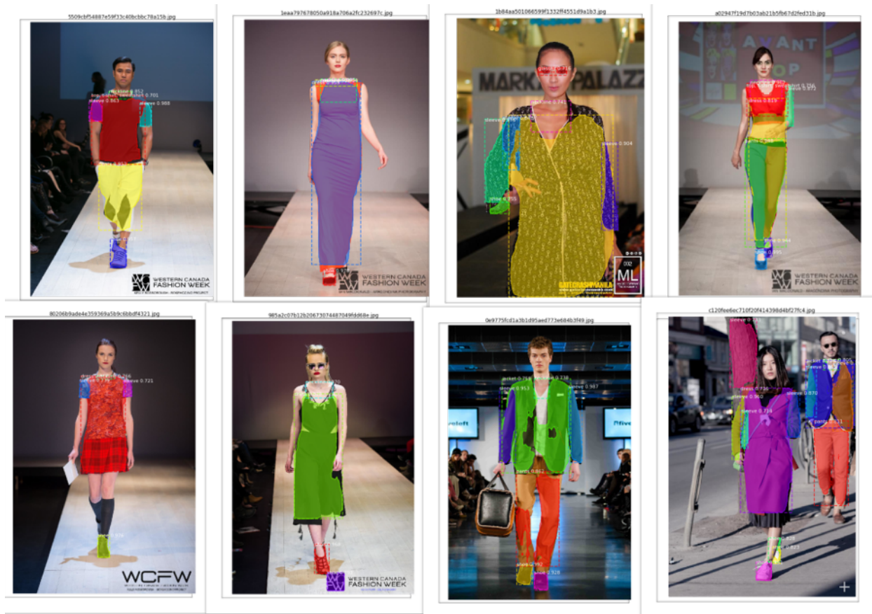
Fig. 5. Predictions from the Mask R-CNN model
