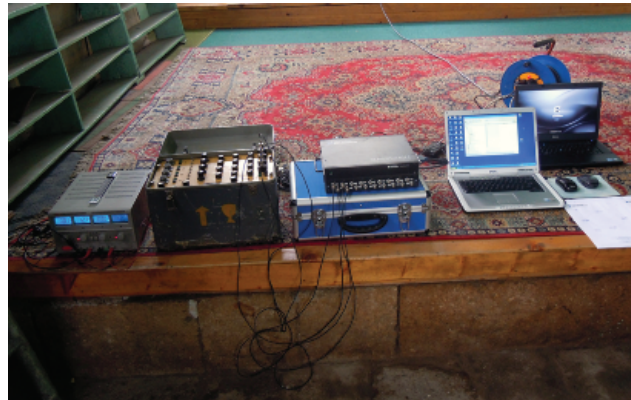
Figure 4: Ambient vibration measurements equipment (Left to right: Power supply, Kinematics SC-1 conditioner, NI DAQPad-6015, Laptops for recording data)
