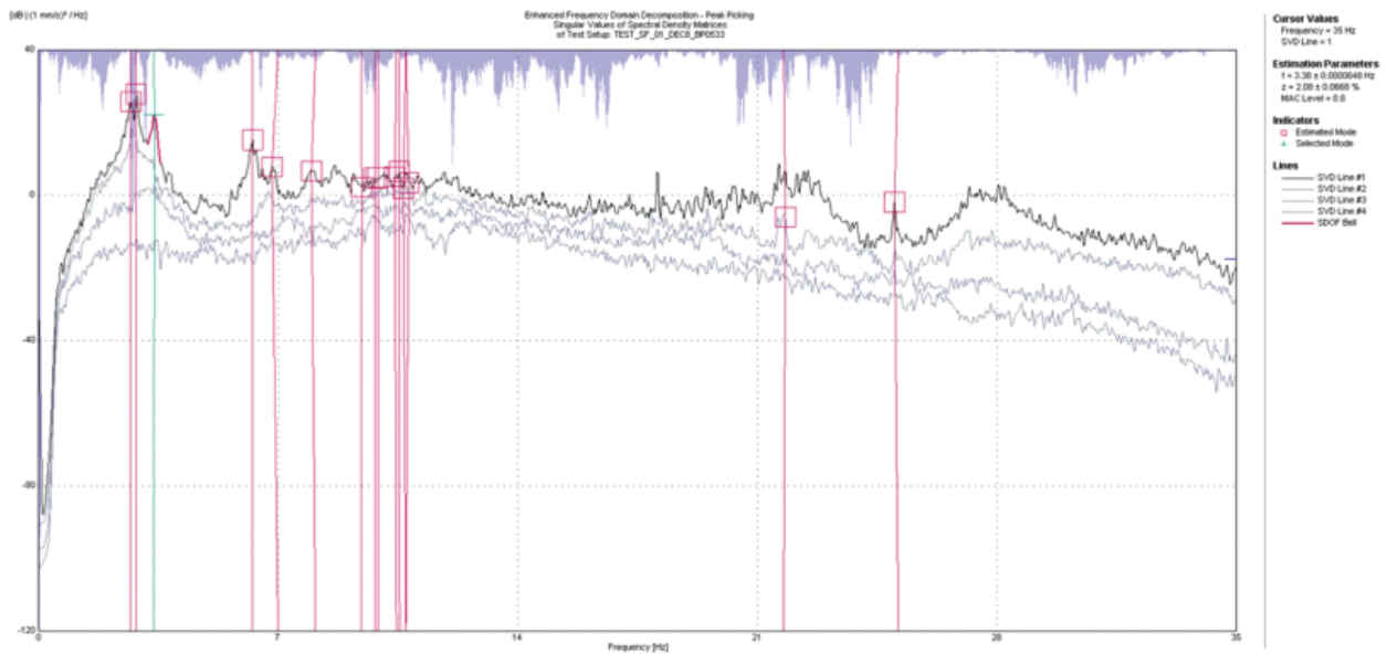
Figure 19: The median of EFDD normalized values of spectral density matrices for all test setups in X and Y directions (2 nd case study)
