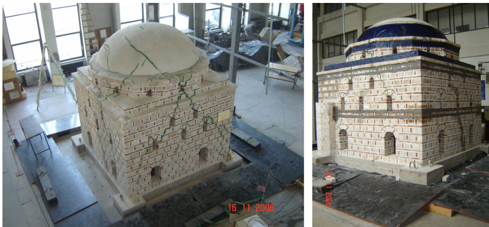
Figure 5. Figure 5a. Mustafa Pasha Mosque - model of original state. Figure 5b. Mustafa Pasha Mosque - model of strengthened state with CFRP bars and wrap.
