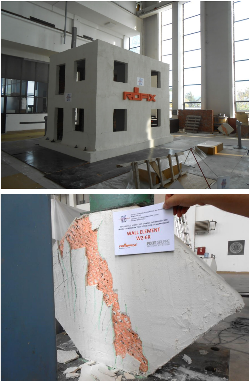
Figure 6 Figure 6a. ROFIX case study - retrofitted model on shaking table. Figure 6b. ROFIX case study - failure mechanisms of strengthened wall element.
