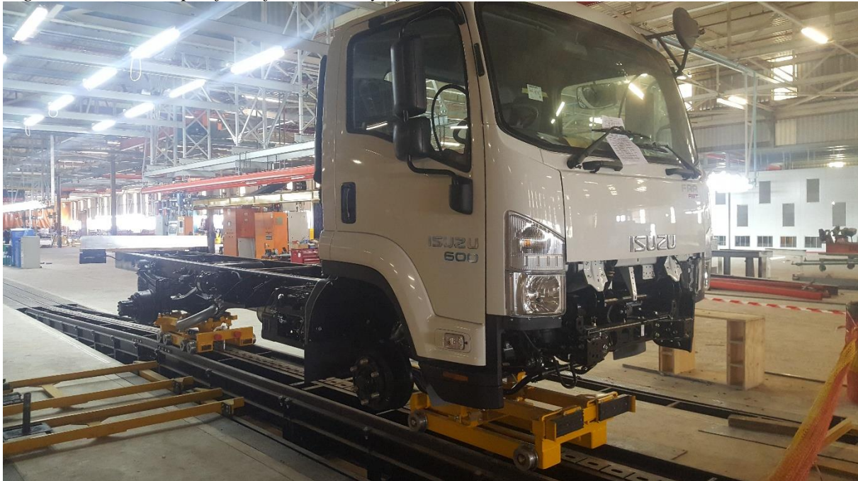
Figure 5: Foldable platform for assembly of trucks
