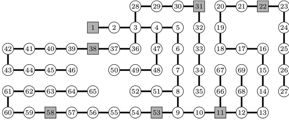
Fig. 5. Topology of 69-node distribution network.
