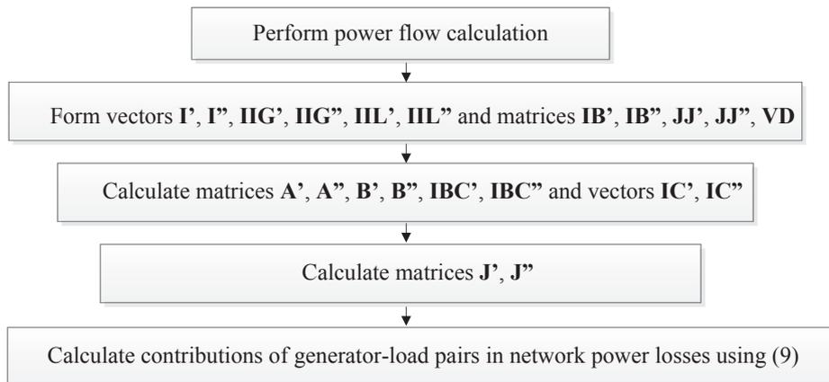
**Fig. 4.** Simple flow-chart of the proposed method.
