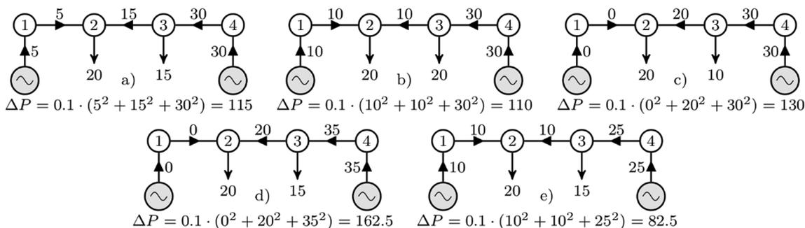
Fig. 6. Changes in power losses due to changes in load and generators currents.
