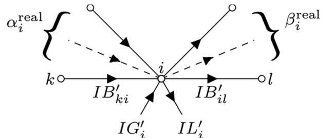
Fig. 3. Real part of currents at node  $i$ .
