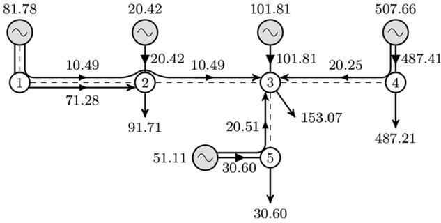
Fig. 2. Real parts of load current components (in amperes).
