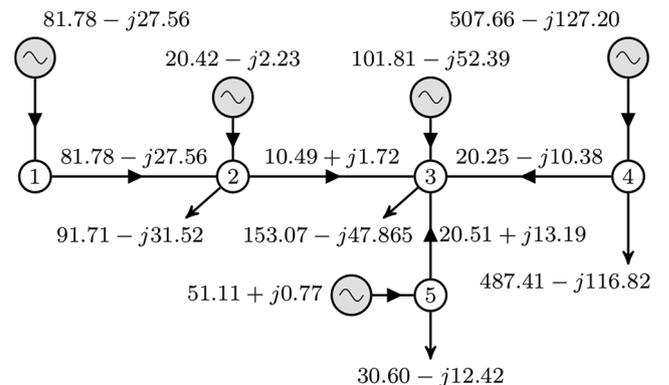
Fig. 1. Simple illustrative example – Complex currents (in amperes).
