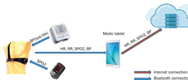
Fig. 4. Transfer of the measured vital data via Bluetooth and via SOAP services.
