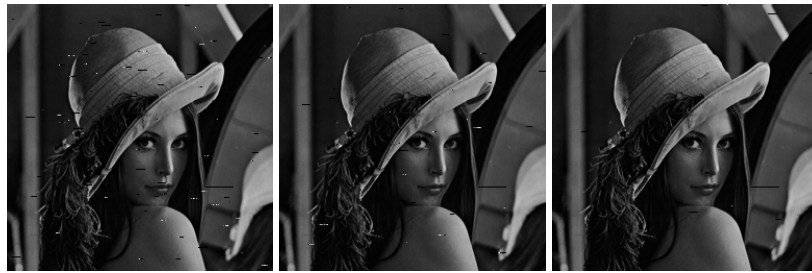
Figure 5.14: Images obtained with Burst-Cut-Decoding algorithm without the filter for P_{GG} = 0.8 , P_{BB} = 0.2
