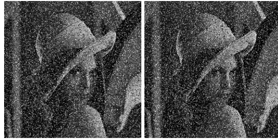
Figure 5.3: Images obtained after transmission through the channel without using any error-correcting code
