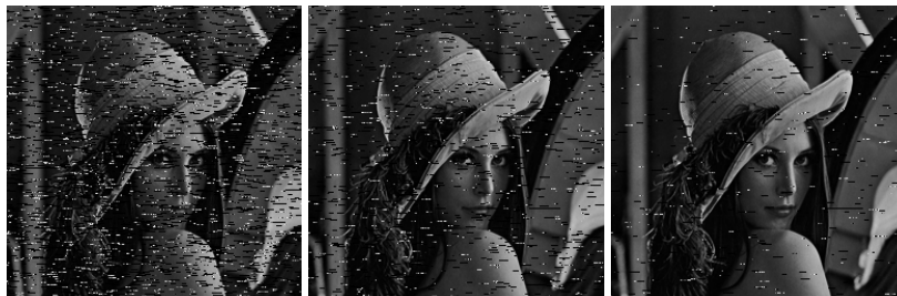
Figure 5.4: Images obtained with Burst-Cut-Decoding algorithm without the filter for P_{GG} = 0.2 , P_{BB} = 0.8
