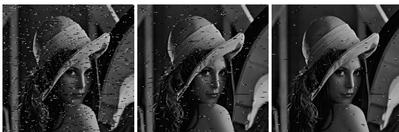
Figure 5.8: Images obtained with Burst-4-Sets-Cut-Decoding algorithm without the filter for P_{GG} = 0.2 , P_{BB} = 0.8
