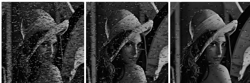
Figure 5.12: Images obtained with Burst-Cut-Decoding algorithm without the filter for P_{GG} = 0.2, P_{BB} = 0.8
