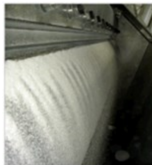
Picture 1: Anhydrous lactose production: Scrape-off and fall into a chute of white DuraLac® H crystals from a rotating drum after spontaneous crystallization on the hot surface.
