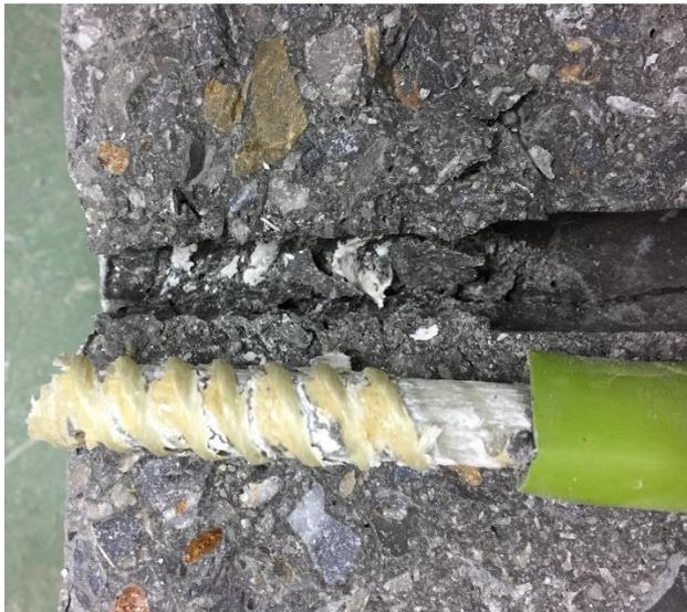
*Figure 22 – Damage on surface of GFRP rebar after pullout testing*
