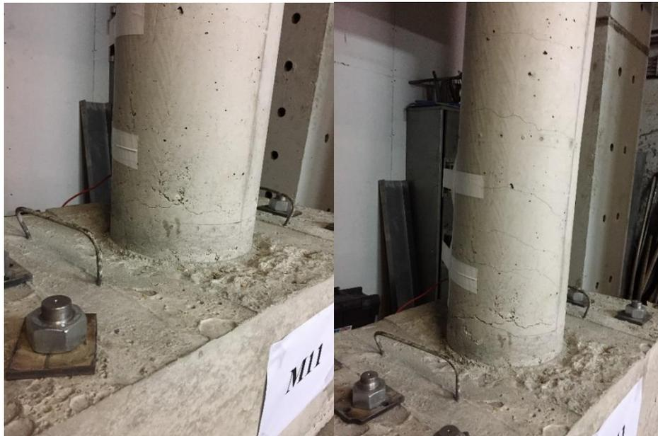
*Figure 4 - Column M11 - Cracking at different stages of loading*
