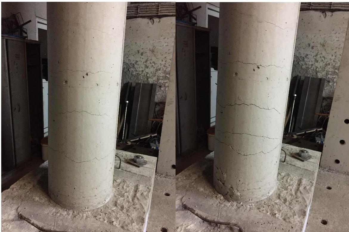
*Figure 14 - Column M21 - Cracking at different stages of loading*
