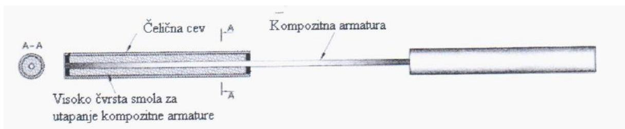
Figure 12 - Testing of GFRP bars in Tension
