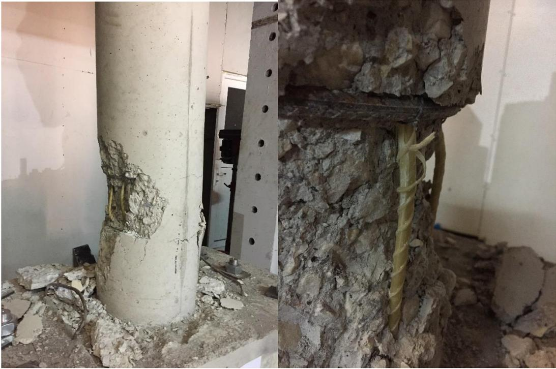
*Figure 21 - Column M31 – Longitudinal Bar buckling and Bond Failure of GFRP rebar*
