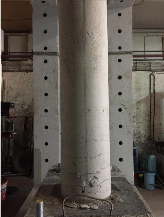
*Figure 24 - Column M32 - Cracking at different stages of loading*
