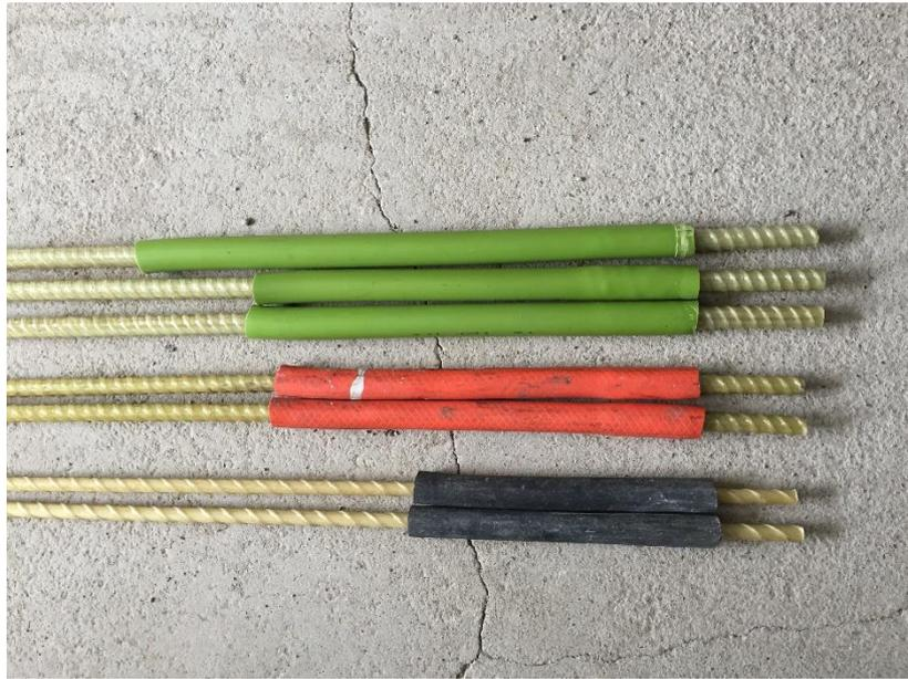
*Figure 19 - Specimens for testing of GFRP and Steel rebar – Isolation of Bars*
