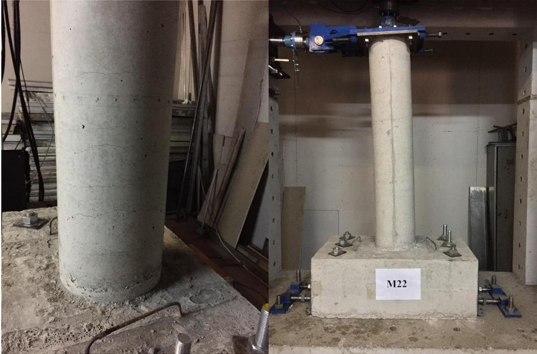
Figure 17 - Column M22 - Cracking at different stages of loading and displacements
