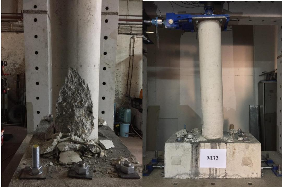
*Figure 25 - Column M32 – Concrete spalling and maximum displaced column*
