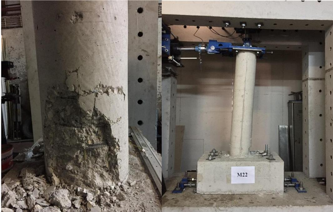
Figure 18 - Column M22 – Cover Spalling and maximum displacement
