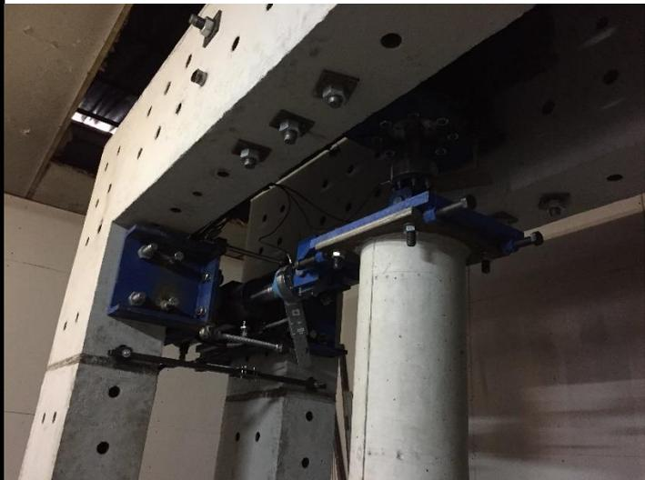
*Figure 23 - Testing frame with installed column and instrumentation*
