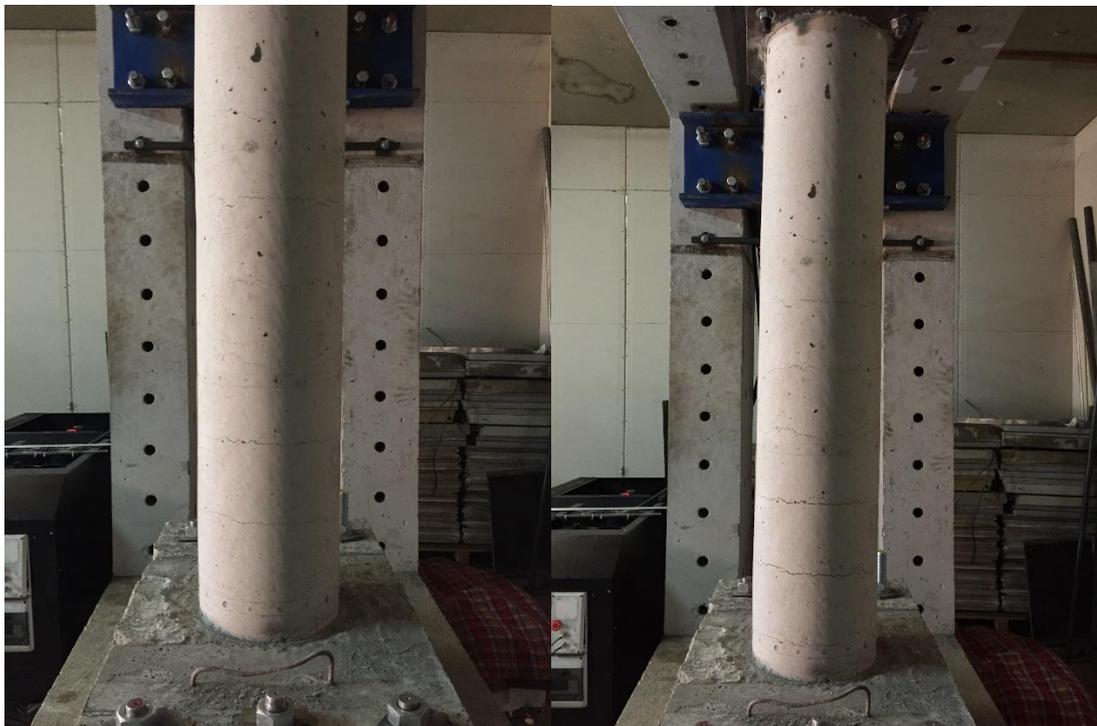
*Figure 20 - Column M31 - Cracking at different stages of loading*
