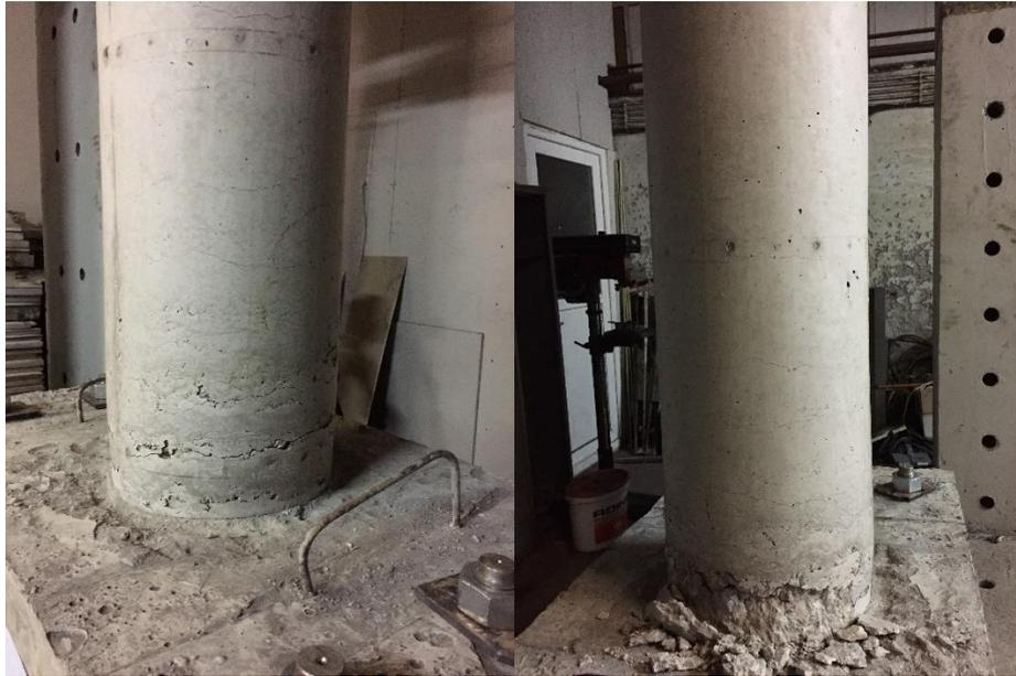
*Figure 7 - Column M12 - Cracking at different stages of loading*
