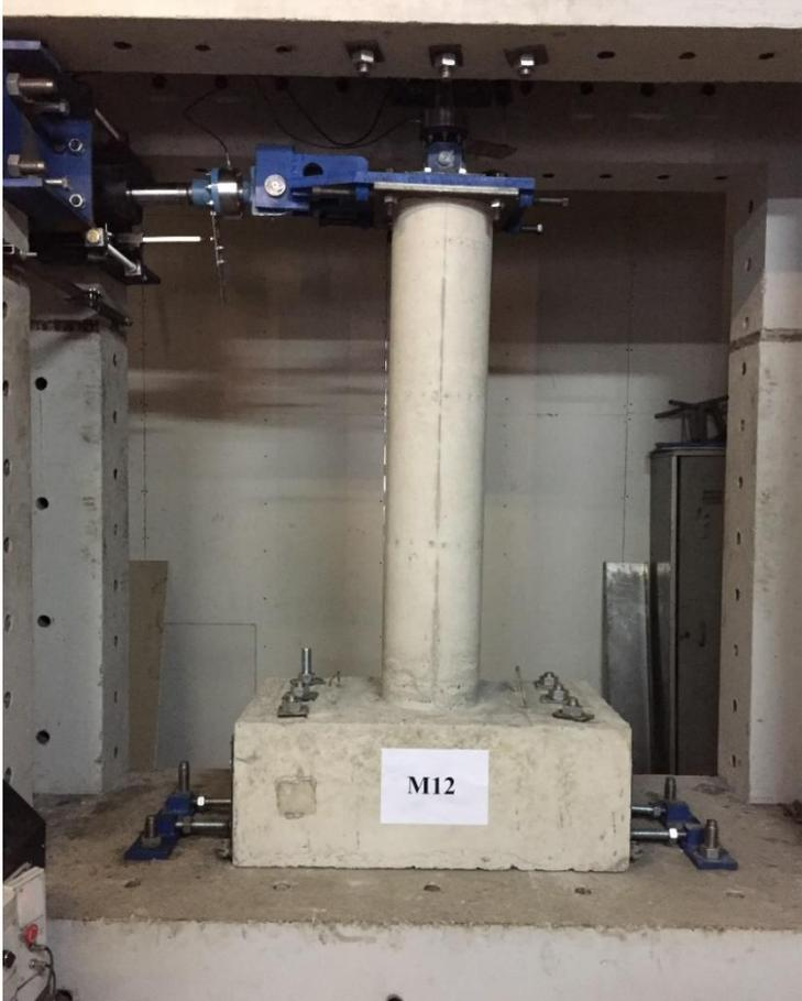
*Figure 6 - Testing of Column M12*
