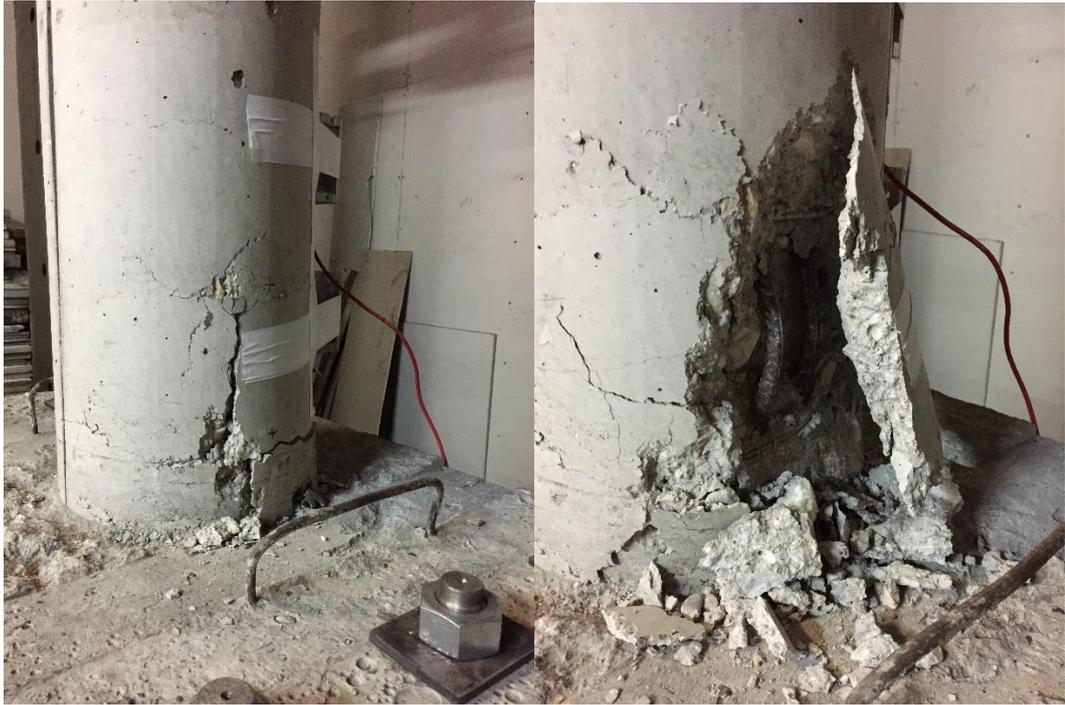
*Figure 5 - Column M11 – Spalling of Cover and Buckling of Longitudinal Rebar*
