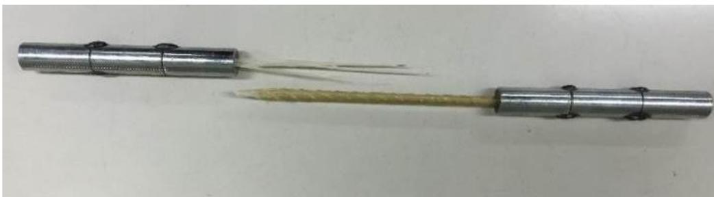
*Figure 10 - Testing of GFRP rebars in tension*
