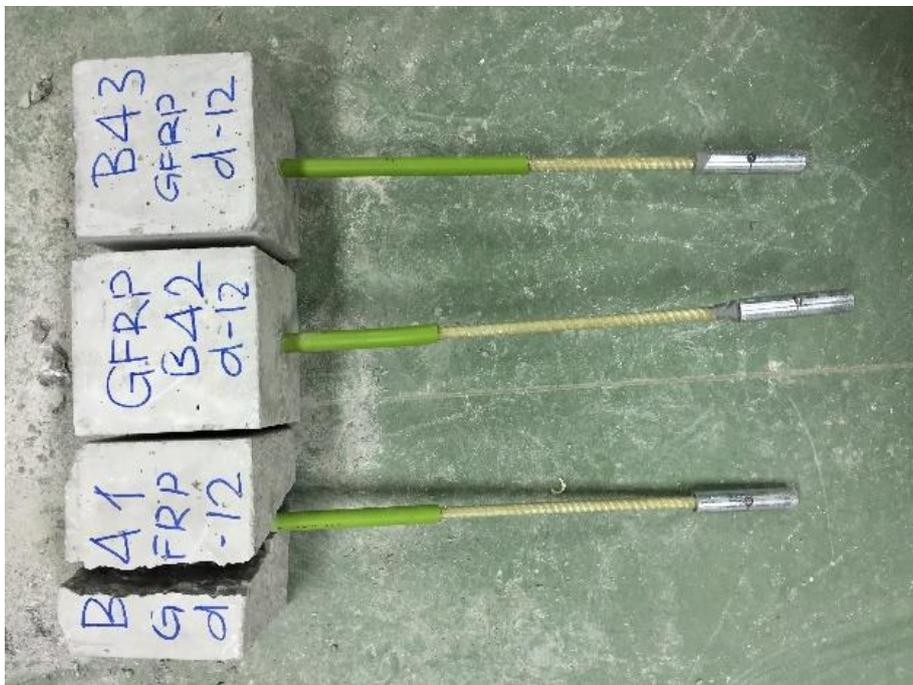
Figure 18 - Specimens for testing of GFRP and Steel rebars – Pull-Out test
