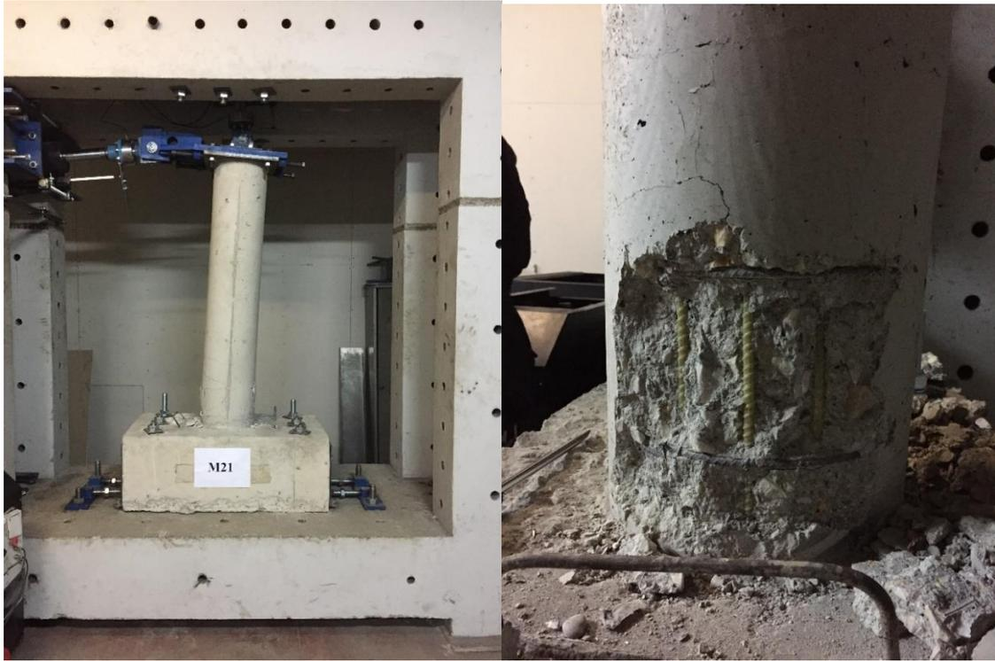
*Figure 15 - Column M21 – Max displacement of column and cover spalling*
