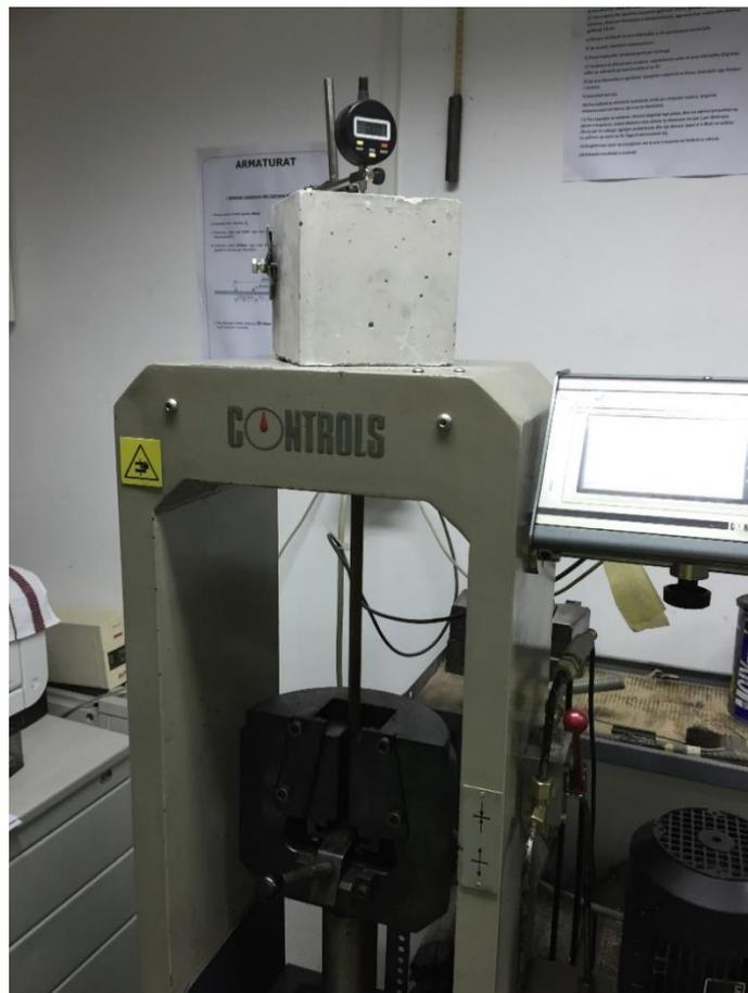
*Figure 20 - Process of Pull out Testing*
