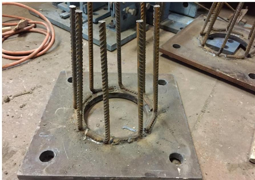
*Figure 7 - Top plate for application of Load*
