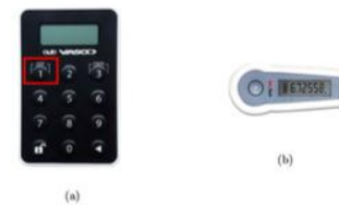
Fig. 3. (a) OTP generator protected by PIN (b) OTP generator not protected by PIN [2]
