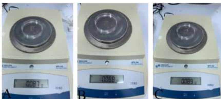
Figure 4: A) Dry weight of the film without Aloe vera gel, B) Dry weight of the film containing 5% gel, C) Dry weight of the film containing 10% gel.
