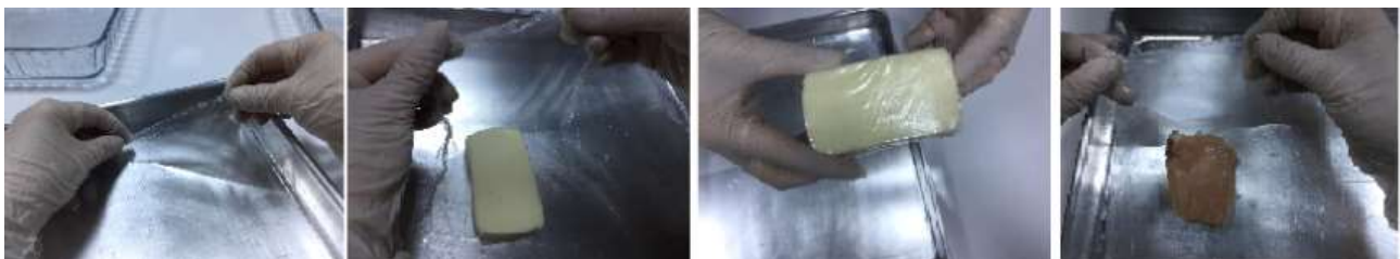
Figure 9: Film produced with PVA only
