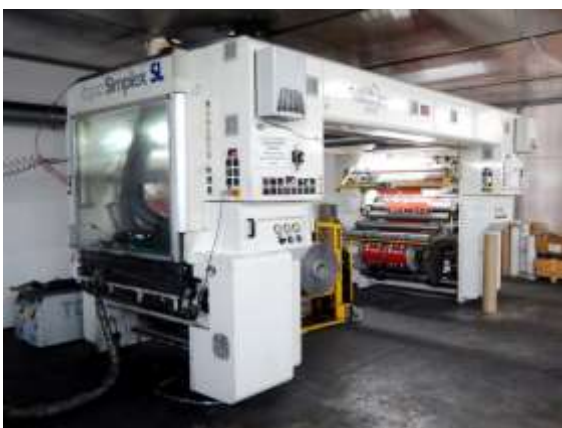
Figure 4. Lamination and slitting processes
