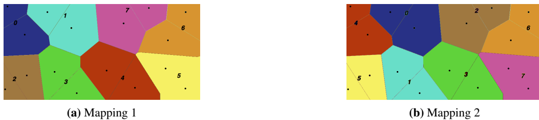
FIGURE 5 Mapping physical coverage area served by two co-located APs to a logical fog community served by 10 edge servers
