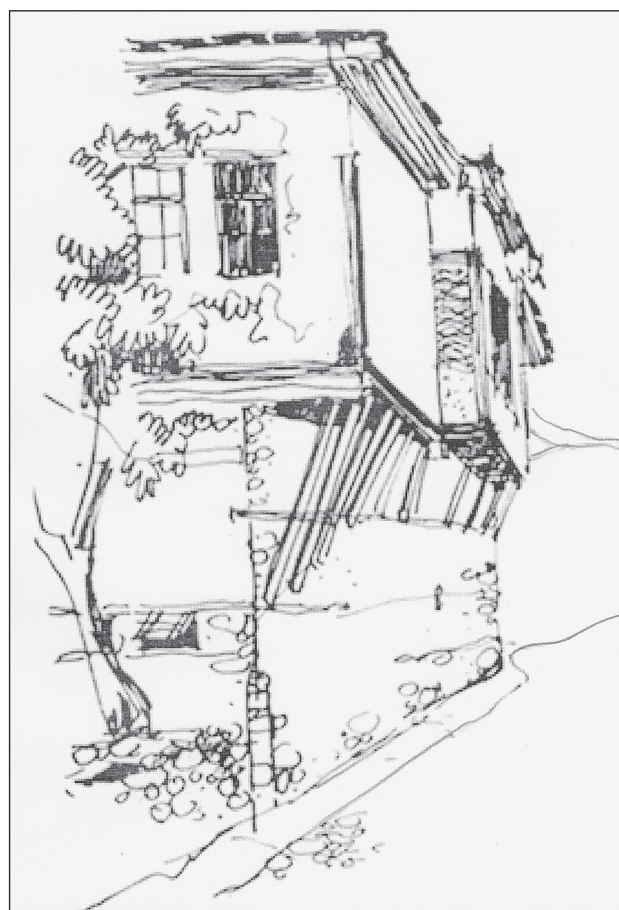
Figure 13. The line of the stony wall at the ground floor directed by the path, is straightened on the upper floors with triangle cantilevered extended supporters. [3]
