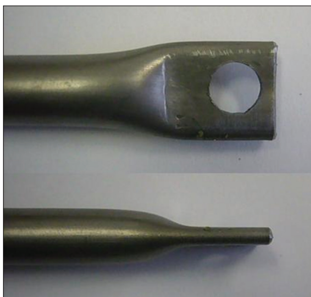
Figure 2. A tube flattening
