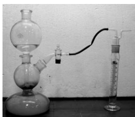
Fig. 2: A Kipp apparatus joined to a wash-bottle via rubber tubing — an example of aesthetic disaster
