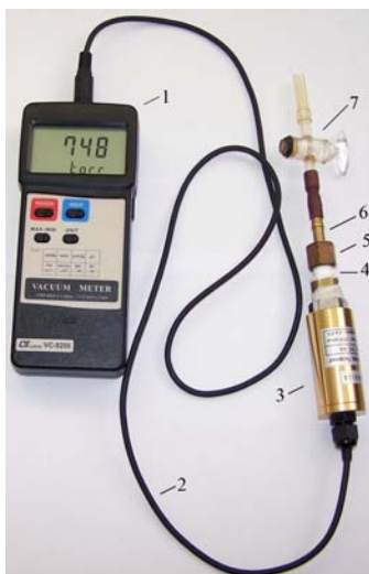
Figure 1. The digital manometer. 1. body of the manometer; 2. connection cable; 3. the pressure gauge; 4. screw covered with teflon tape; 5. nut; 6. brass inlet/outlet tube; 7. glass tube with a stopcock.
