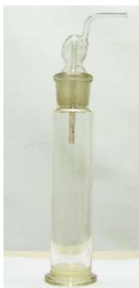
Figure 2. The reaction chamber used for the determination of the oxygen content of air.
