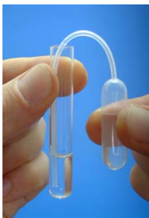
Figure 2. Filling the plastic pipet with a solution.
