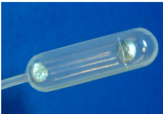
Figure 4. Inserting Zn granules into the plastic pipet.
