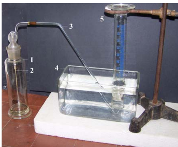
Figure 1. Experimental setup for the reaction of sodium metal with water vapor (1 – a wash-bottle used as a reaction chamber; 2 – iron spoon; 3 – doubly bent glass tube; 4 – pneumatic trough; 5 – graduated cylinder).
