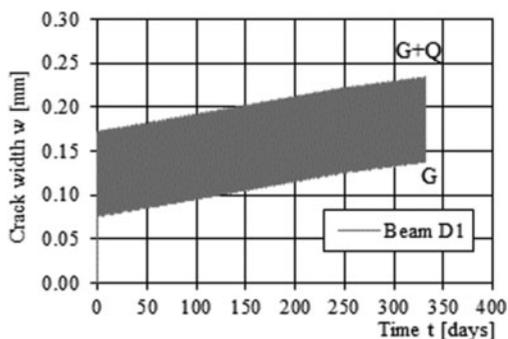
Figure 6. Diagram crack width  $w$  – time  $t$  for beam D1 concrete class C30/37.
