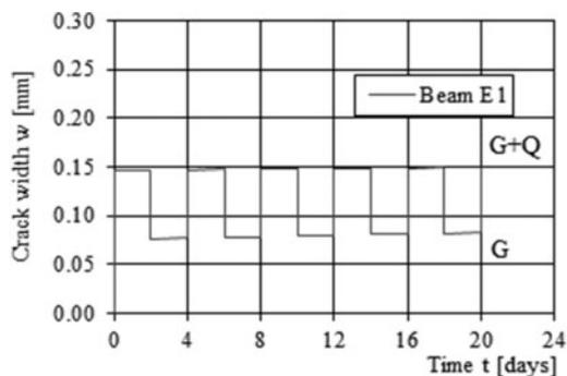
Figure 5. Diagram crack width  $w$  – time  $t$  for beam E1 concrete class C30/37.
