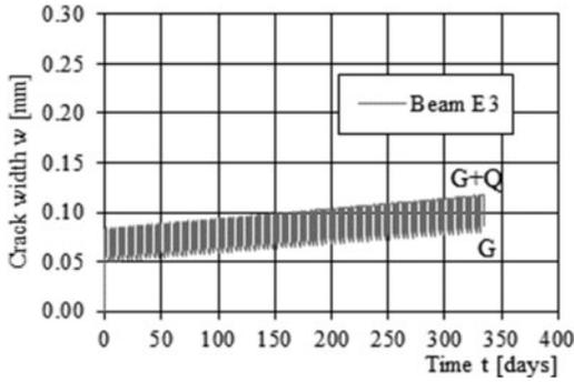
Figure 9. Diagram crack width  $w$  – time  $t$  for beam E3 concrete class C60/75.
