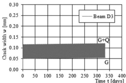
Figure 7. Diagram crack width  $w$  – time  $t$  for beam D3 concrete class C60/75.
