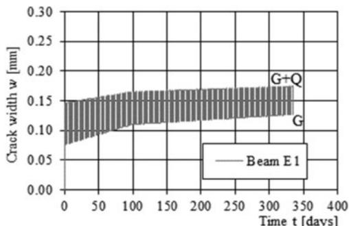
Figure 8. Diagram crack width  $w$  – time  $t$  for beam E1 concrete class C30/37.
