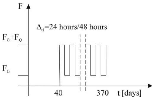
Figure 3. Loading history for the elements of series D and E.
