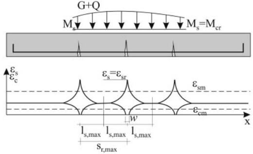
Figure 2. Stabilized cracking phase.
