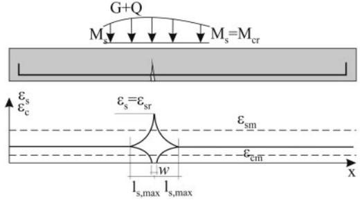
Figure 1. Crack formation phase.
