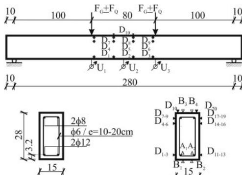
\*D-mechanical deformer, A-strain gauge for reinforcement, B-strain gauge for concrete, U-deflection-meter
