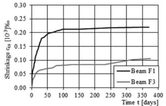
Figure 10. Diagram shrinkage  $\varepsilon_{cs}$  – time  $t$  for beam F1 concrete class C30/37 and for beam F3 concrete class C60/75.
