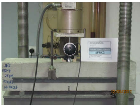
Figure 2: Testing of flexural tensile strength and concrete creep
