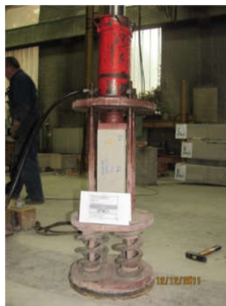
Figure 2: Testing of flexural tensile strength and concrete creep
