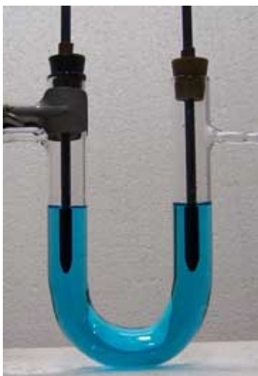
Figure 1. The setup for the electrolysis of \text{CuSO}_4(\text{aq}) .
