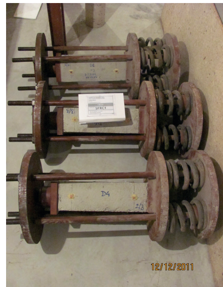
Fig. 2 Testing of concrete creep in creep frames
