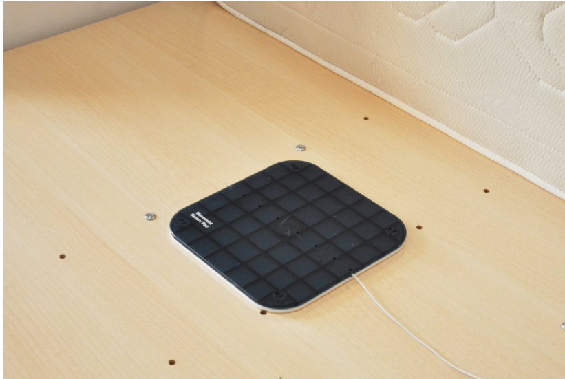
Figure 1. Piezoelectric based bed movement sensor under mattress
