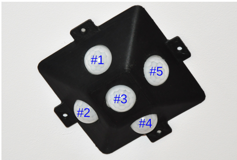
Figure 2. Sensor module with PIR sensors
