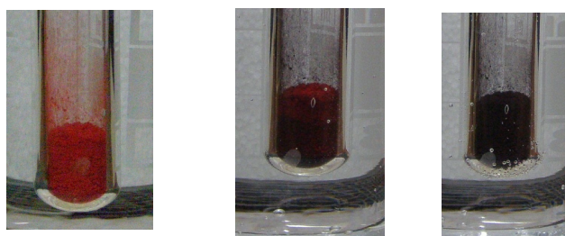
Figure 3. Remarkable colour change in \text{Cu}_2[\text{HgI}_4] . Leftmost photo – room temperature; the rest are at \square 80^\circ\text{C} (the longer the heating, the more complete the colour change)
