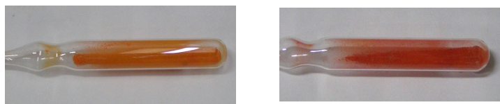
Figure 4. Noticeable colour change in solid solution (\text{Ag, Cu})[\text{HgI}_4] . Left – room temperature; right – high temperature
