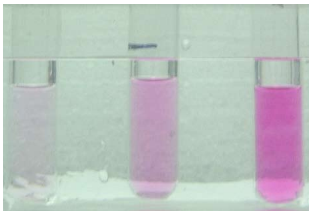
Figure 1: The colour of phenolphthalein in 4 mol/L (left), 2 mol/L (middle) and 1 mol/L (right) solutions of NaOH, immediately after the indicator was added
