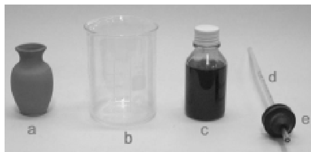
Figure 2. Equipment used for demonstration of effusion in liquids: porous cup (a); beaker (b); bottle filled with colored glycerol (c); graduated glass tube (d); one hole rubber stopper (e).
