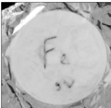
Figure 5. Marks on filter paper soaked with potassium hexacyanoferrate(II), written with iron and copper anode
