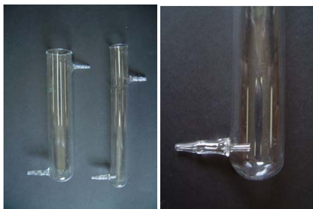
Figure 1. (left) Flow chambers for demonstration experiments (two variants). (right) Enlarged photograph of the inlet tube used for bubbling a gas through a liquid (see Figure 1a, right chamber).
