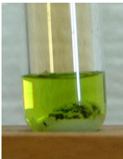
Figure 7. Copper grain in fuming nitric acid containing traces of water (photographed after several days). The white powder is Cu(NO 3 ) 2 and the dark covering on the grain is possibly CuO.
