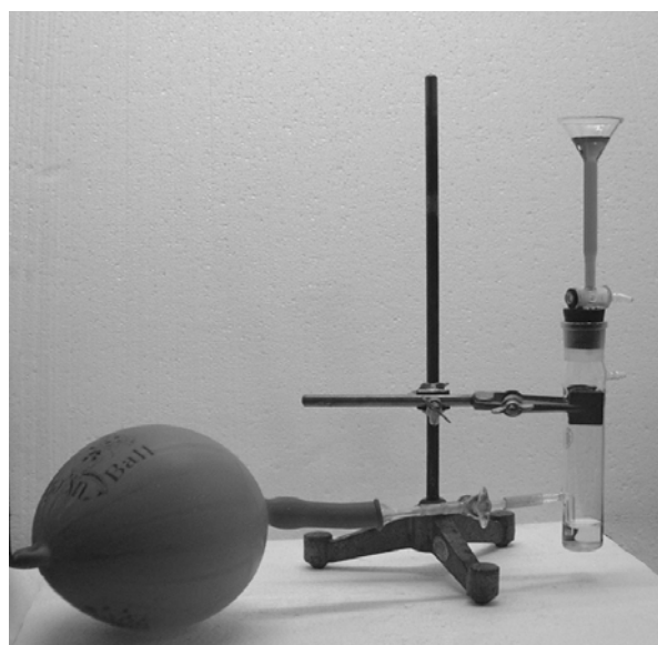
Fig. 2. Setup for demonstration of the free radicals' properties: (left) balloon filled with oxygen or nitrogen; (right) purpose built reaction chamber, partly filled with benzene solution containing triphenylmethyl (on the top of the chamber is the separation funnel containing benzene solution of iodine)
