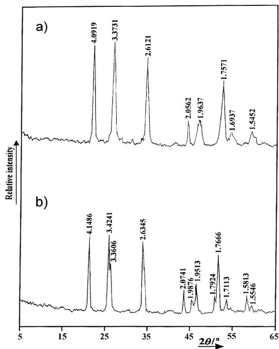
Fig. 4. X-ray powder diffraction patterns of residues obtained following isothermal treatment at: (a) 400°C; (b) 600°C.
