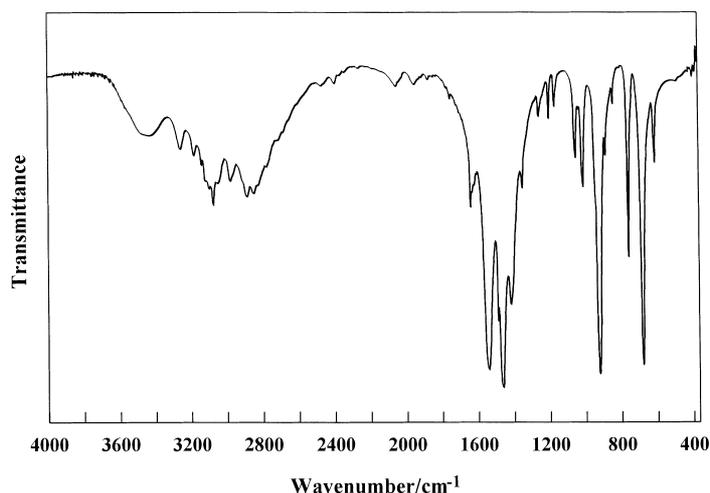
Fig. 1. FTIR spectrum of pyridinium uranyl acetate.
