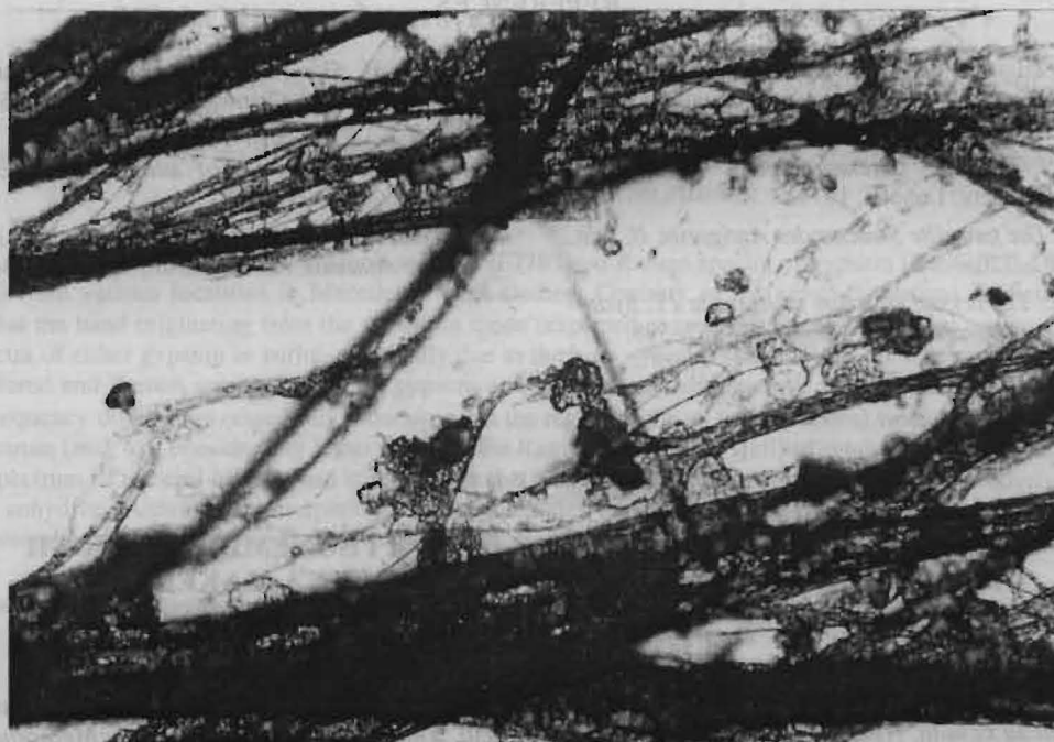
Fig. 6. Microscopic aggregates of serpentine mineral chrysotile (Mob. 20 X H +)
