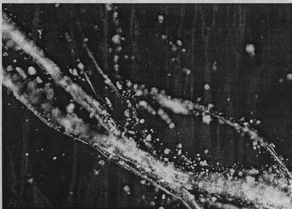
Fig. 1. Microscopic aggregates of serpentine mineral chrysotile (Mob. 20 X H +)
