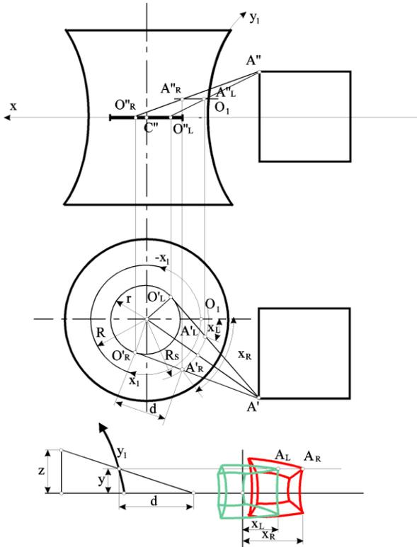
Figure 1. Method for developing stereometric projections of a cube in a hyperboloid space
