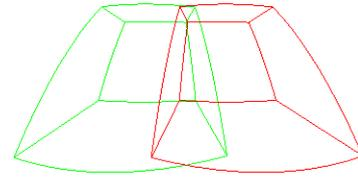
Figure 8. Stereometric projections of a cube in a paraboloid projective space.
