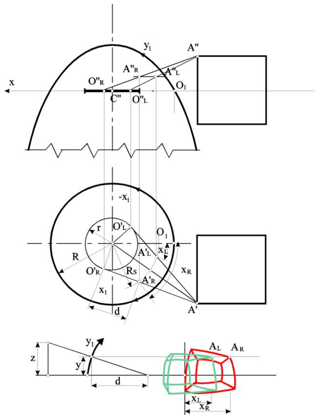
Figure 3. Method for developing stereometric projection of a cube in a paraboloid projective space
