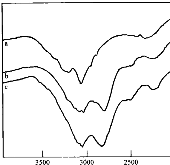
Fig. 1. The O-H stretching region of the spectra of [\text{Cu}(\text{bpy})]\text{BeF}_4 \cdot 2\text{H}_2\text{O} (a), [\text{Cu}(\text{bpy})]\text{SO}_4 \cdot 2\text{H}_2\text{O} (b) and [\text{Cu}(\text{bpy})]\text{SeO}_4 \cdot 2\text{H}_2\text{O} (c)
