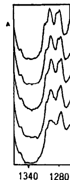
Fig. 3. The N-D bending region in the spectra of slightly deuterated \text{ApTS}
