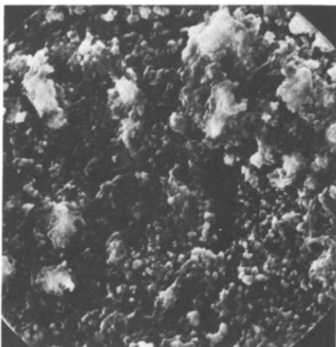
Fig. 1. Scanning electron micrograph of a ZnO thin film. (Magnification 4500 ×.)
