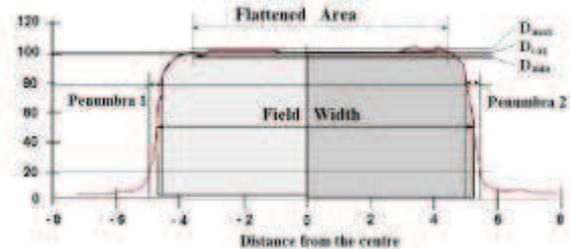
Fig. 3 – Definition of flattened area of a beam profile
